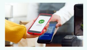
NFC (Near Field Communication) is a specific version of passive HF RFID primarily used for contactless consumer transactions, such as payments and ticket confirmations. NFC also works on the basis of radio signals, but only at a very short distance, for example, when someone makes a payment by holding a bank card or smartphone within a few centimetres of a reader. Another strength of NFC is the possibility to guide people to additional information using their smartphone.
