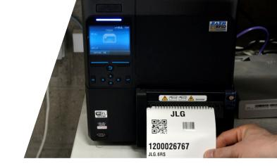
RFID labels can be printed via the POLARIS website or via the handheld. An RFID printer is specifically designed to write data on the RFID chips embedded in RFID labels. Very useful if
