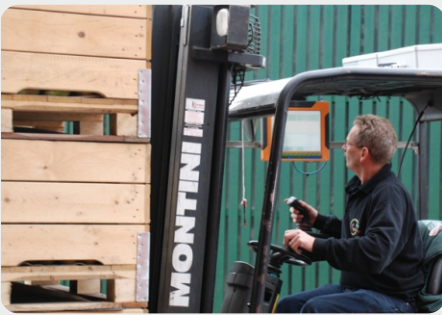
forklift truck equipped with RFID readers and a Windows terminal
