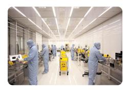
A clean room is an environment, typically used in manufacturing or scientific research, designed to reduce or exclude environmental pollutants.
