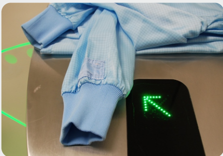
Aucxis determined the right position of the laundry tag on the cleanroom clothing for optimal scanning.
