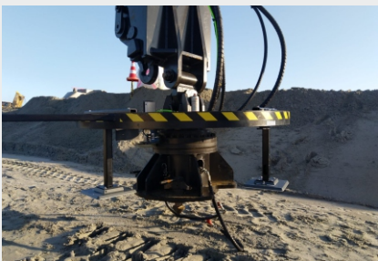
Installation of RFID antennas and readers on pontoon crane.
