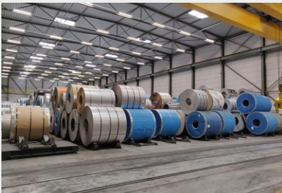
Rolls of stainless steel, ready to be reprocessed into cut-to-size steel plates.
