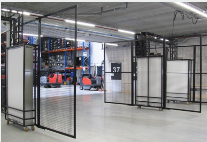
The Aucxis RFID gates were modulated by Rent-All into mobile registration gates.
