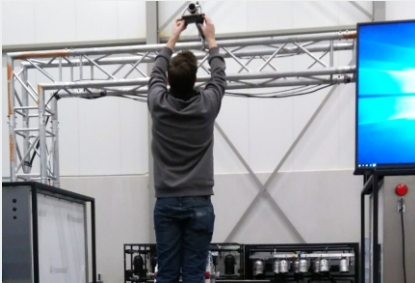
Mounting of the mobile RFID UHF gate with sensors for starting and stopping the scanning.
