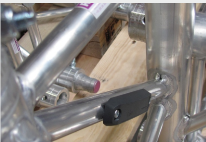
Specifically for the identification of the trusses, preference was given to an elongated, long-range on-metal tag.
