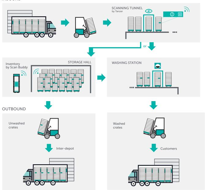
RFID enables to monitor the flow of the pallets from inbound to outbound to the auctions or to other depots.
