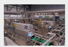
In the washing station, the RFID label is scanned, allowing EPS to know how many and which types of crates are ready for delivery.
