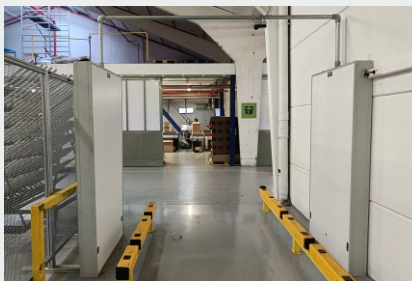
This RFID gate registers which boots are located on which cart enabling the packing manager to plan everything smoothly and correctly.
