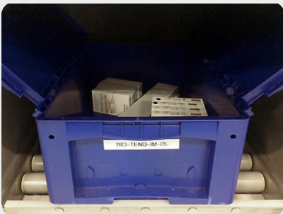
An implants bin can be easily rolled into the RFID scan box.
