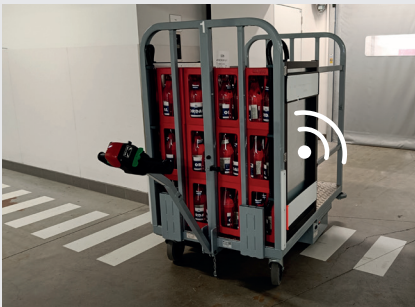
Mobile RFID equipment, integrated in the existing logistic trolleys
